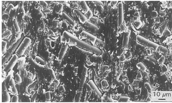
Figure 8 Surface features after disruption of the thin film, at 0.04 slip ratio, 300 N normal load and 1000 r.p.m. running speed; direction of friction from bottom to top.
